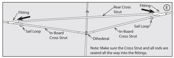
**Step 6:** Insert Rear Cross Strut into Fitting on the In-Board Cross Strut. (diagram E)
